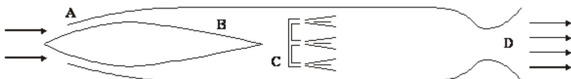
When moving at high speed, air enters the nose at **A** and its pressure increases up to region **B**. At **C**, fuel is injected directly into the air stream where it is ignited, and the burning gases are exhausted at high speed through the nozzle at **D**. This provides the thrust.
